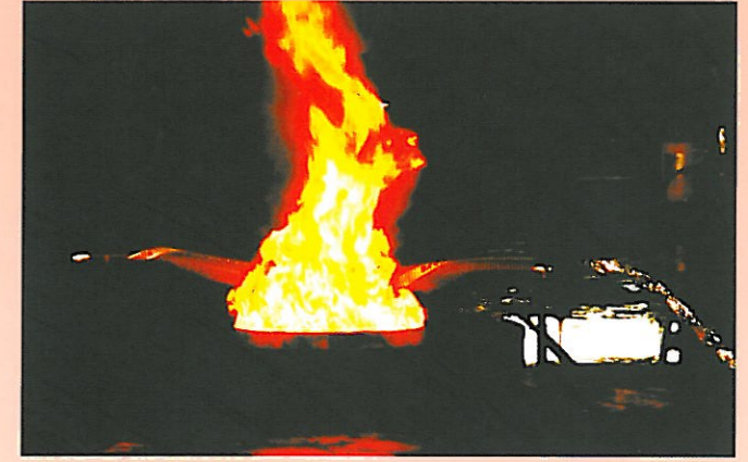
HOSE FULL OF PRODUCT UNDER EXTREME FIRE ATTACK.
